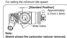
NOTE: While the Mixture Control Valve and the Metering Valve are set at the standard position when the engine leaves the factory, readjustment may be necessary, occasionally to allow for changes in fuel formula and climatic conditions Readiust the controls only when satisfactory results cannot be obtained with the standard positions following the instructions mentioned in the "CARBURETOR ADJUSTMENT" section.
