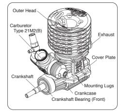
The engine is installed with a 0.1mm thick and a 0.15mm thick gasket for 25% nitro fuel when it leaves the factory. Adjust the total thickness according to atmospheric temperature, humidity and glowplug used.
