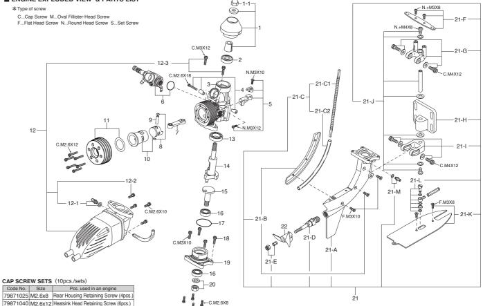
Code No. Size Pcs. used in an engine 79871025 M2.6x8 Rear Housing Retaining Screw (4pcs.) 79871040 M2.6x12 Heatsink Head Retaining Screw (6pcs.) 79871055 M2.6x18 Carburetor Retainer Retaining Screw (1pc.
