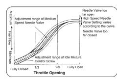
NOTE: With this carburetor, neither the Idle Mixture Control Screw adjustment, nor the Medium Speed Needle Valve adjustment will have any effect on mixture strength when the throttle is fully (or almost fully) open.
