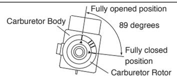
When the triangle mark on the carburetor rotor meets the far right mark, the throttle is fully closed. When the triangle mark meets the top mark, the throttle is fully open. The range is 89 degrees. You may use the other three marks as the reference marking of throttle opening to your preference when hovering.
