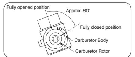
As shown in the sketch, the carburetor has graduation marks. When the triangle mark on the carburetor rotor meets the most right mark, throttle is fully closed. When the triangle mark meets the top mark, throttle is fully open. The range is approximately 80 degrees. You may use other three marks as the reference marking of throttle opening to your preference when hovering.
