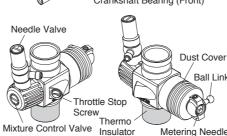
■ CARBURETOR CONTROLS • STANDARD POSITIONS (POSITIONS WHEN THE ENGINE LEAVES THE FACTORY)
