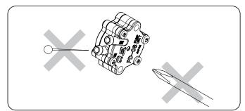
■ DO NOT obstruct the small rectangular hole at the bottom of the regulator, nor the regulator will not function correctly.
