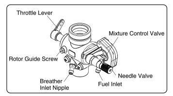
Two mixture controls are provided on this Carburetor.
