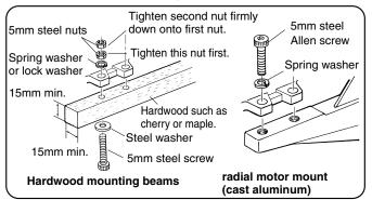
Make sure that these mounting beams are accurately aligned and firmly integrated with the airframe, reinforcing the adjacent structure to absorb vibration. Use 5mm or larger steel screws, preferably Allen type hexagon socket head cap screws, with washers and locknuts, for bolting the engine to the bearers.
