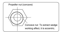
There is a risk, particularly with powerful fourstroke engines, of the propeller flying off if the prop nut loosens due to detonation ("knocking") in the combustion chamber when the engine is operated too lean, or under an excessively heavy load.
