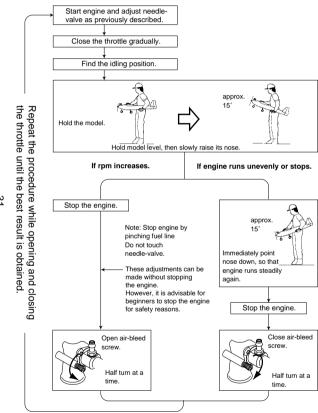
Attention: Do not leave the glowplug connected to the battery while adjusting the carburetor throttle.
