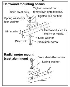
Make sure that these mounting beams are accurately aligned and firmly integrated with the airframe, reinforcing the adjacent structure to absorb vibration. Use 3mm or larger steel screws, preferably Allen type hexagon socket head cap screws, with washers and locknuts, for bolting the engine to the bearers.
