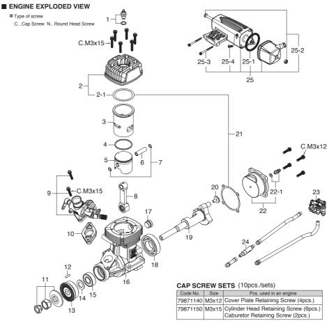
Description 1 27881400 Throttle Lever Assembly 1-1 22081313 Throttle Lever Retaining Screw 2 28181210 Carburetor Rotor 3 28181600 Mixture Control Valve Assembly "O" Ring (L) (2pcs.) 3-1 28181920 3-2 28181910 "O" Ring (S) (2pcs.) 4 28181110 Carburetor Body 5 45581820 Roter Guide Screv 6 28181950 Universal Nipple No.17 7 28181900 Needle Valve Assembly 7-1 28181970 Needle Assembly 7-2 26381501 Set Screw "O" Ring (2pcs.) 7-3 28181910 7-4 27381940 Needle-valve Holder Assembly Ratchet Spring No.4
