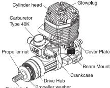
Crankshaft Propeller washer
