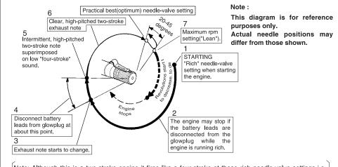
Note: Although this is a two-stroke engine it fires like a four-stroke at these rich needle-valve settings-i.e. ignition of the fuel charge takes place at every fourth stroke of the piston instead of at every second stroke.
