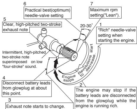
Note: Although this is a two-stroke engine it fires like a four-stroke at these rich needle-valve settings-i.e. ignition of the fuel charge takes place at every fourth stroke of the piston instead of at every second stroke.
