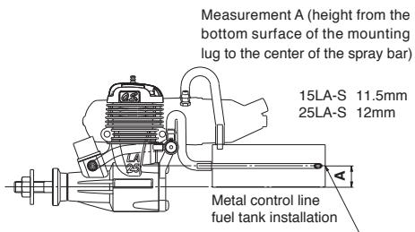
Make sure that the center of the spray bar and tank are on the same line.
