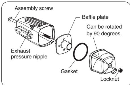
■ **In case of installing the silencer direct to the engine**
