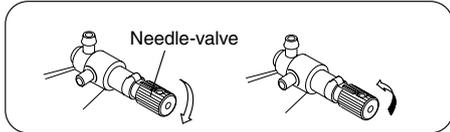
The position where the needle-valve stops is the fully closed position. It may be convenient to remember the position of the mark or set-screw at this time.
