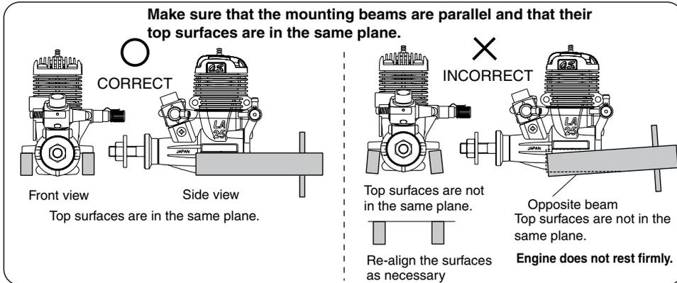
**How to fasten the mounting screws.**
