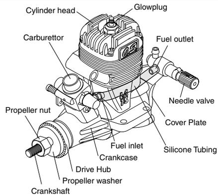
Connect the short length of fuel tubing supplied securely between the fuel outlet and the fuel inlet. In the event of the tubing becoming damaged, it should be replaced with a suitable length of best quality 5mm ODX2mm ID silicone tubing. Use similar material to connect the fuel inlet nipple to the fuel tank.
