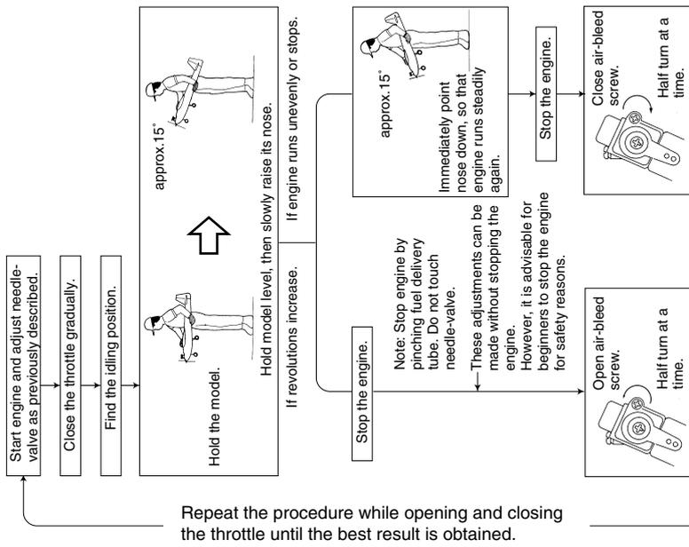
Repeat the procedure while opening and closing the throttle until the best result is obtained.
