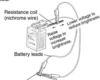
Adjust applied voltage by changing the position of clip on resistance coil until glowplug element is glowing bright red.
