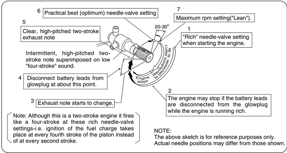
On starting from cold, with the needle-valve set at the rich starting position:
