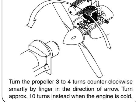
Turn the propeller 3 to 4 turns counter-clockwise smartly by finger in the direction of arrow. Turn approx. 10 turns instead when the engine is cold.
