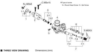
Description 1 27881400 Throttle Lever Assembly 1-1 22081313 Throttle Lever Retaining Screw 2 28181210 Carburetor Rotor 3 28181600 Mixture Control Valve Assembly "O" Ring (L) (2pcs.) 3-1 28181920 3-2 28181910 "O" Ring (S) (2pcs.) 4 28181110 Carburetor Body 5 45581820 Roter Guide Screv 6 28181950 Universal Nipple No.17 7 28181900 Needle Valve Assembly 7-1 28181970 Needle Assembly 7-2 26381501 Set Screw "O" Ring (2pcs.) 7-3 28181910 7-4 27381940 Needle-valve Holder Assembly Ratchet Spring No.4
