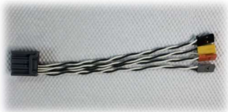
【PWM signal harness】 •It is used to input each signals of throttle, fuel trim, starter and ignition on/off by PWM signals from RC receiver, etc. It is not used when connecting to S.BUS or RS485.
