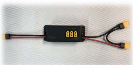
【Power distribution box with a fuse】Model : HUB-01 •Distribution box with a fuse for SGC. •Connect two 6 cell li-po batteries with capacity of 3000mAh or more to 2 pieces of XT60(F). There is no balance charging function. Must use two batteries in same condition. *For connection details, refer to the SGM(Starter Generator Motor) section in this manual.
