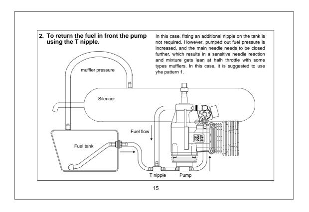
The pump requires running-in as with the engine. Be sure to check the silicone tubes and connections carefully for any cracks on the tubes and loose connections as the engine runs ejecting excess fuel.
