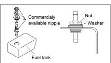
Clear the burr, if any, off the hole to fit the nipple with a cutter knife. Also clean the tank with methanol to remove the dust or tank cut-off particle.
