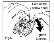
6. If clearance is correct, loosen the locknut on the other rocker-arm and repeat steps 1 to 5 above. Finally, replace rocker box cover.
